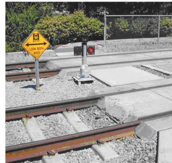
Figure 4-29. “Low-Rise” Pedestrian signal in use in Portland, Oregon. Source: FRA Compilation of Pedestrian Safety Devices in Use at Grade Crossings.
