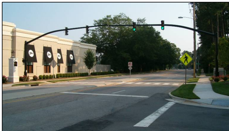
Figure 4-5. Examples of pedestrian-activated, signalized, mid-block crossings.
