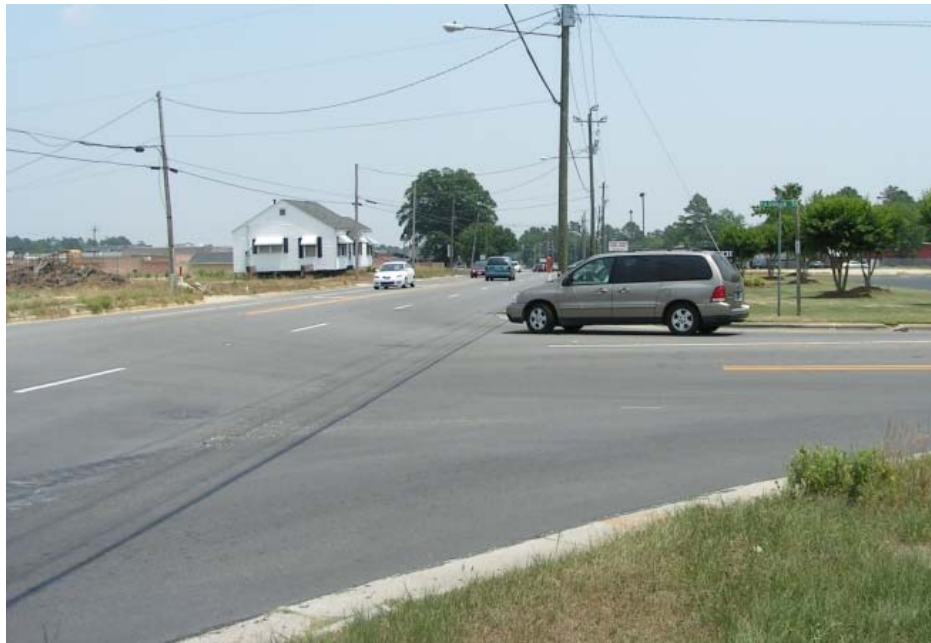
Figure 5-10. This photograph illustrates the wide curb radius at the Erwin Rd and Tilghman Rd intersection. The images to the right illustrate possible treatments including a curb extension and high-visibility crosswalk (top), or a combination of the curb extension treatment with a textured asphalt crosswalk and median refuge island for added pedestrian safety and comfort (bottom).
