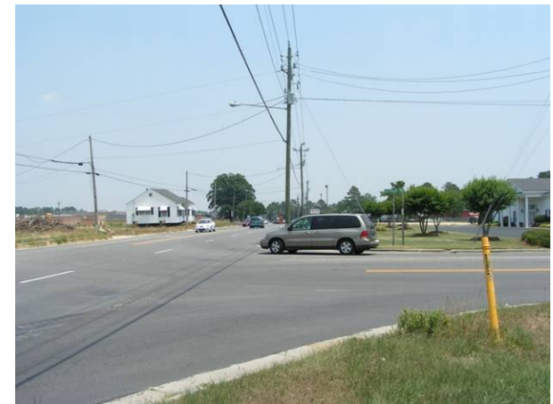
Figure 5-6 (below) Intersection of Erwin Road and Tilghman Road. Wide corners or "curb radii" at intersections can encourage high-speed right-turning movements and create wider crossing distances for pedestrians at intersections. Intersection treatments called "curb extensions" can help create a safer environment for pedestrians in these instances.
