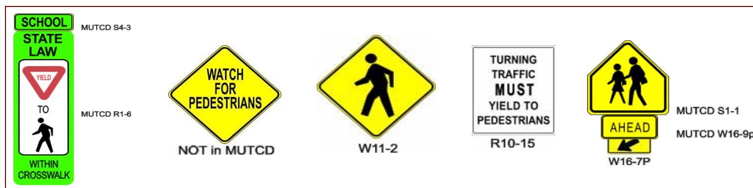
Figure 4-12. Example standard pedestrian warning signs. The first sign (far left) is usually installed within the street to warn motorists to yield to pedestrians in a crosswalk - it does not have to be near a school. The second and third signs are common general pedestrian warning signs, while the fourth and fifth signs notify motorists of specific instances to watch for pedestrians. The fourth sign, "Turning Traffic", is usually placed at intersections to warn motorists that are turning right or left to yield to pedestrians in crosswalks. For the fifth sign, the top sign can either be combined with the smaller "ahead" sign or the arrow symbol to indicate the presence of a crosswalk to motorists in a school zone.
