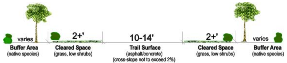
Figure 4-14. Example cross-section for a typical greenway.
